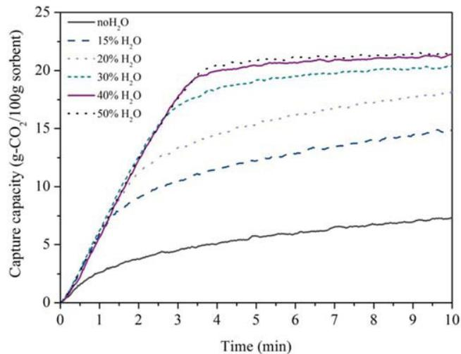
Fig. 2. CO<sub>2</sub> uptake profiles with 15 vol % CO<sub>2</sub> (with 0 - 50 vol % H<sub>2</sub>O, balanced in N<sub>2</sub>) at 898 K.
