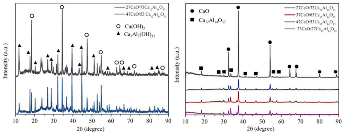
Fig. 1. (a) X-ray diffraction patterns of two different as-synthesized dried hydrothermal sorbents:  $\circ$   $\text{Ca}(\text{OH})_2$ ,  $\blacktriangle$   $\text{Ca}_3\text{Al}_2(\text{OH})_{12}$ ; (b) X-ray diffraction patterns of calcined hydrothermal (1273 K, 1 h) sorbents with different  $\text{CaO}/\text{Ca}_{12}\text{Al}_{14}\text{O}_{33}$  ratios:  $\bullet$   $\text{CaO}$ ,  $\blacksquare$   $\text{Ca}_{12}\text{Al}_{14}\text{O}_{33}$ .
