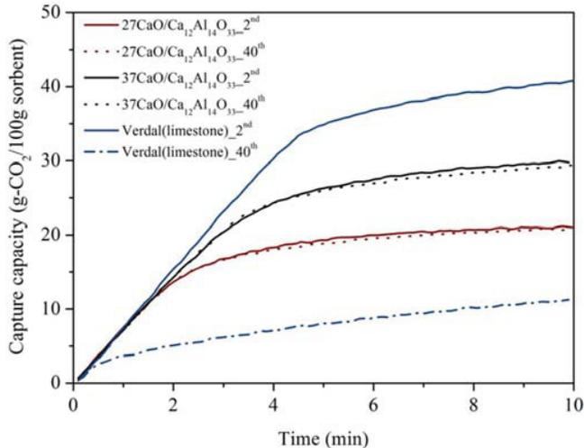
Fig. 4. CO<sub>2</sub> uptake profiles under pre-combustion condition: Carbonation: 873 K for 10 min, 15 vol % CO<sub>2</sub>, 47 vol % H<sub>2</sub>O, balanced in N<sub>2</sub>.
