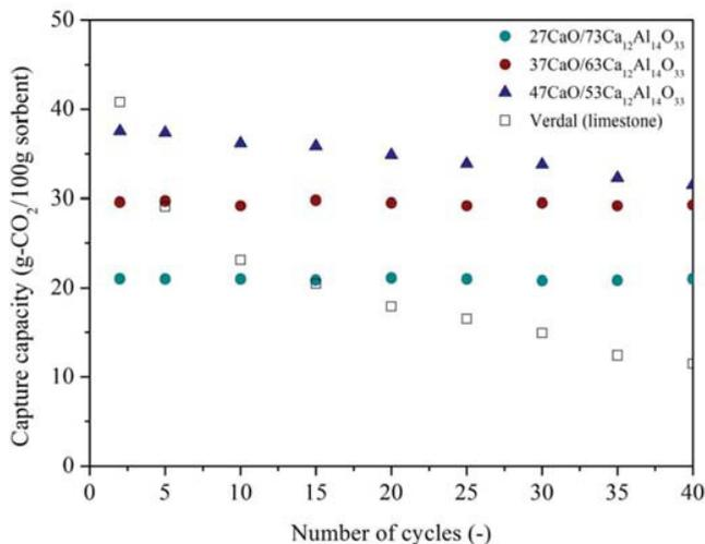
Fig. 3. CO<sub>2</sub> capture capacity of synthetic and natural sorbents over 40 cycles under pre-combustion condition. Carbonation: 873 K for 10 min; 15 vol % CO<sub>2</sub>, 47 vol % H<sub>2</sub>O balanced in N<sub>2</sub>. Regeneration: 21 vol % CO<sub>2</sub>, 78 vol % H<sub>2</sub>O, balanced in N<sub>2</sub>, 1123 K for 3 min. Verdal limestone is included as reference.
