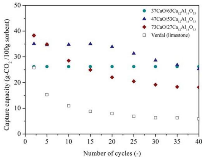
Fig. 5. CO<sub>2</sub> capture capacity of synthetic and natural sorbents during 40 cycles under post-combustion condition. Carbonation: 923 K for 10 min; 14.5 vol % CO<sub>2</sub>, 13 vol % H<sub>2</sub>O balanced in N<sub>2</sub>. Regeneration: 100 vol % CO<sub>2</sub>, at 1193 K for 3 min). Verdal limestone is included as reference.
