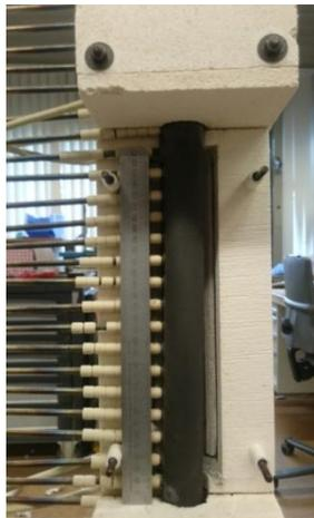
Figure 2 Packed bed reactor setup at TU/e lab
