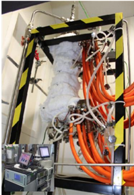
Figure 2 Spouted bed at the laboratories of the Imperial College of London
