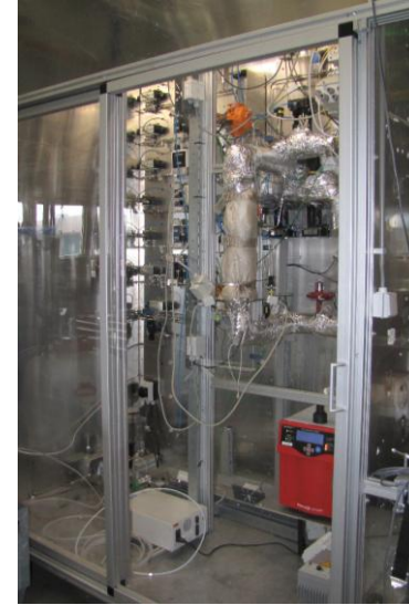
Figure 3 Fixed bed test rig at the ECN lab for testing sour conditions
